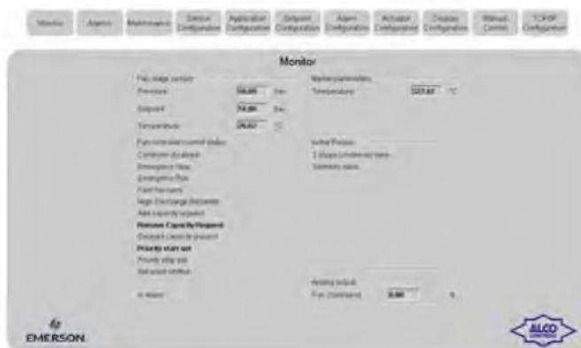
The **TCP/IP based Controllers** offer a practical solution, particularly for smaller installations that require communication for monitoring purposes without the need for customized visualization. For many installations, an additional monitoring server is not required.
